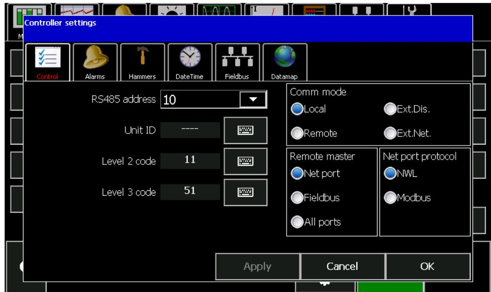
For Local operation, press the *Local* button in the **Comm mode** box of the **Control** tab
