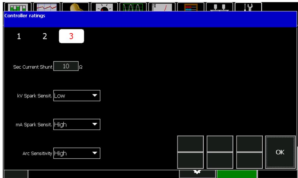
**Sec Current Shunt:** This is the value of the mADC feedback resistor that is used to measure the T/R output current. It can be located in either the T/R junction box or in the control enclosure.
