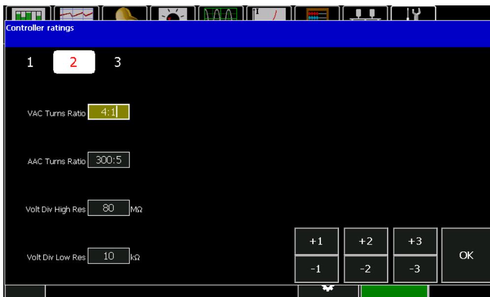
**VAC Turns Ratio:** This is the ratio of the primary metering transformer being used to measure the primary voltage at the T/R set. This transformer is usually located in the control enclosure.
