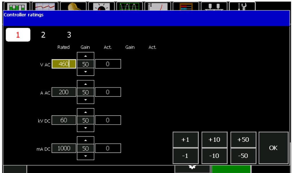
This screen shows the electrical ratings for the unit. These ratings must be correct to allow the control to maintain operation within safe values.
