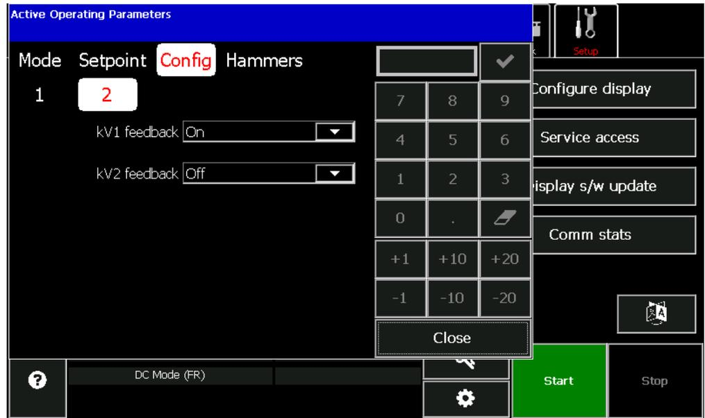
If the T/R set being controlled is a double-half wave unit, or has no provision for KV feedback, you will have to select the settings that accurately describe the configuration.
