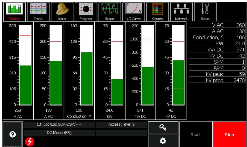
1. V AC displays the primary voltage of the T/R set.
