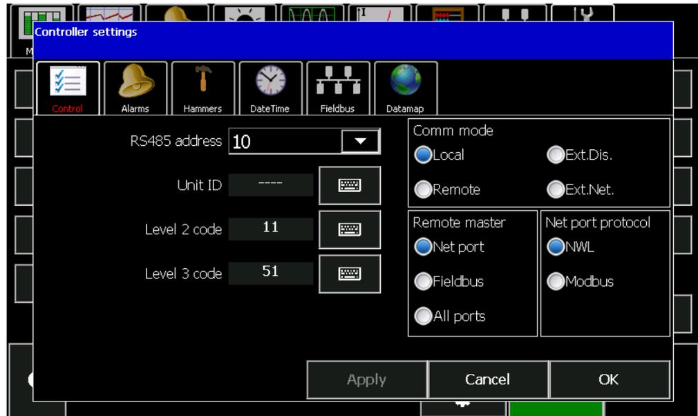
When you set the **Comm mode** for a GVC to local or remote in the **Setup** you will not have full access to all GVC functions. Some are compatible with both local and remote control, but others are exclusive to one or the other. The table below shows the breakdown by mode.
