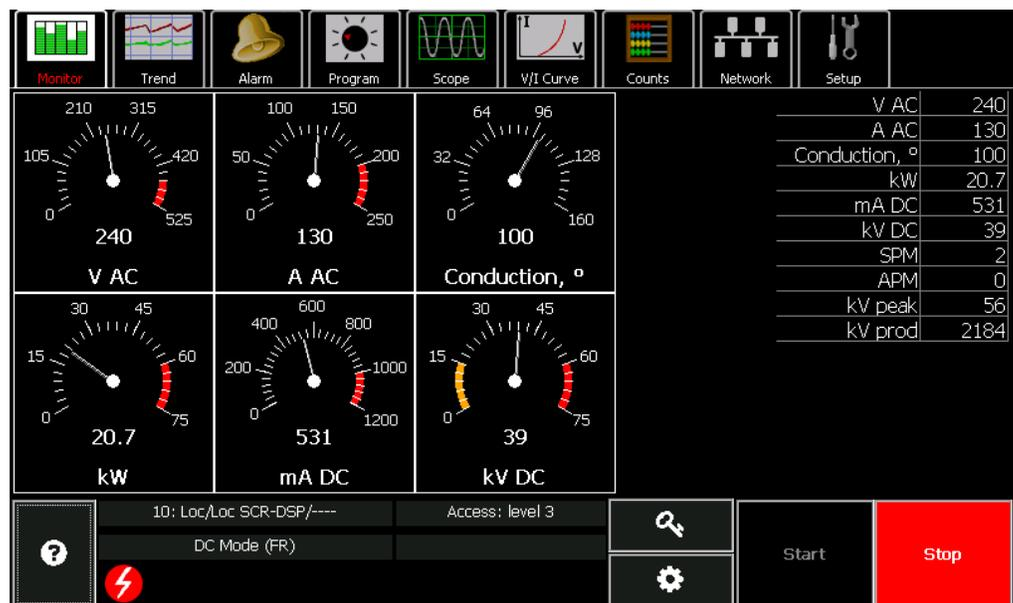
The red portion of the meters indicate operation at values that are exceeding the rating of the unit. The orange portion of the kVDC meter indicates operation below the UV trip point.
