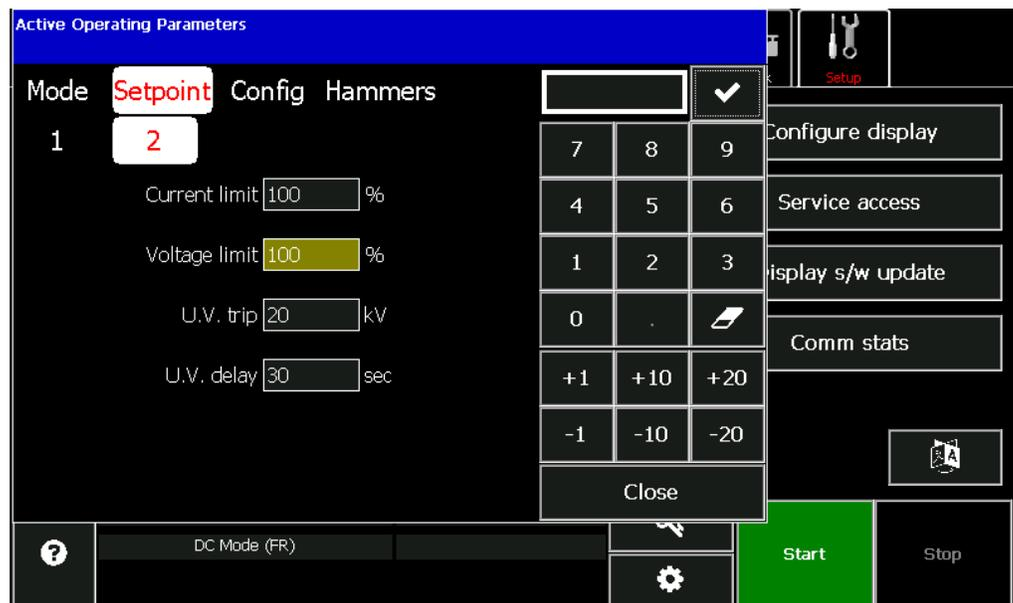
Highlight the U.V.Trip parameter value by touching it. Using the keypad on the right side of the screen press 0 and then press the
