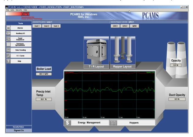
PCAMS consists of a main I/O interface, LCD module, PC with monitor, keyboard, mouse, and proprietary software (Microsoft Windows<sup>®</sup> OS based) for ESP equipment control, data logging, trending, energy management and display.
