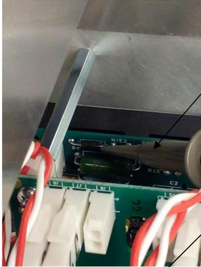
Connect probe to D4 diode as shown for IGBT B, D, E, G, J, L, M, & O. The rightmost column of boards are oriented as shown with D4 at the top. The leftmost column of boards are turned upside-down, so D4 is on the bottom.
