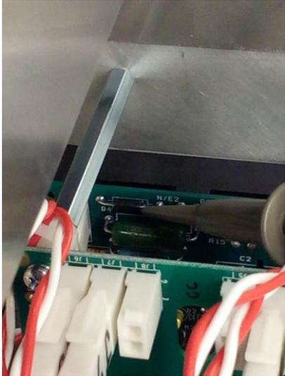
Connect probe to D4 diode as shown for IGBT B, D, E, & G.
