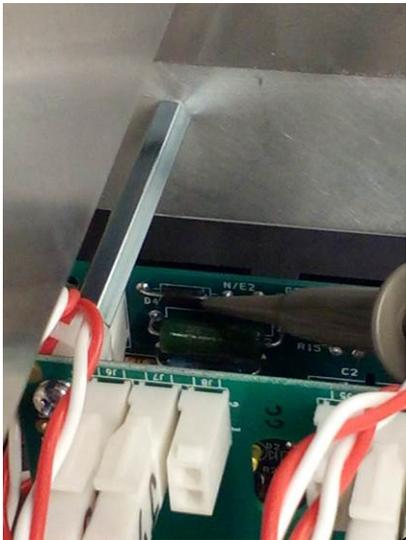
Connect probe to D4 diode as shown for IGBT B & C.
