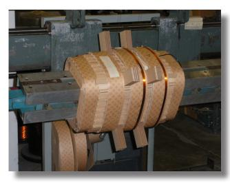
As a fully certified ISO 9001:2000 facility, our Bordentown, NJ factory winds coils (above), builds diode boards, and fabricates all subassemblies in-house.
