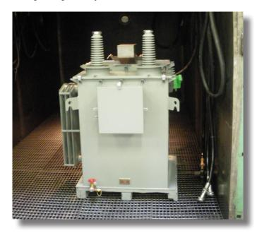
NWL has two oil processing chambers that allow the high voltage tanks to be filled under a strong vacuum, ensuring the windings are totally impregnated.
