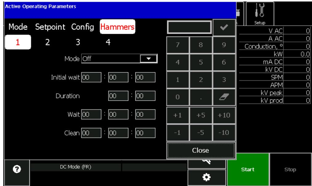
There are four screens, one for each rotating hammer output. Below is a definition list of the parameters.
