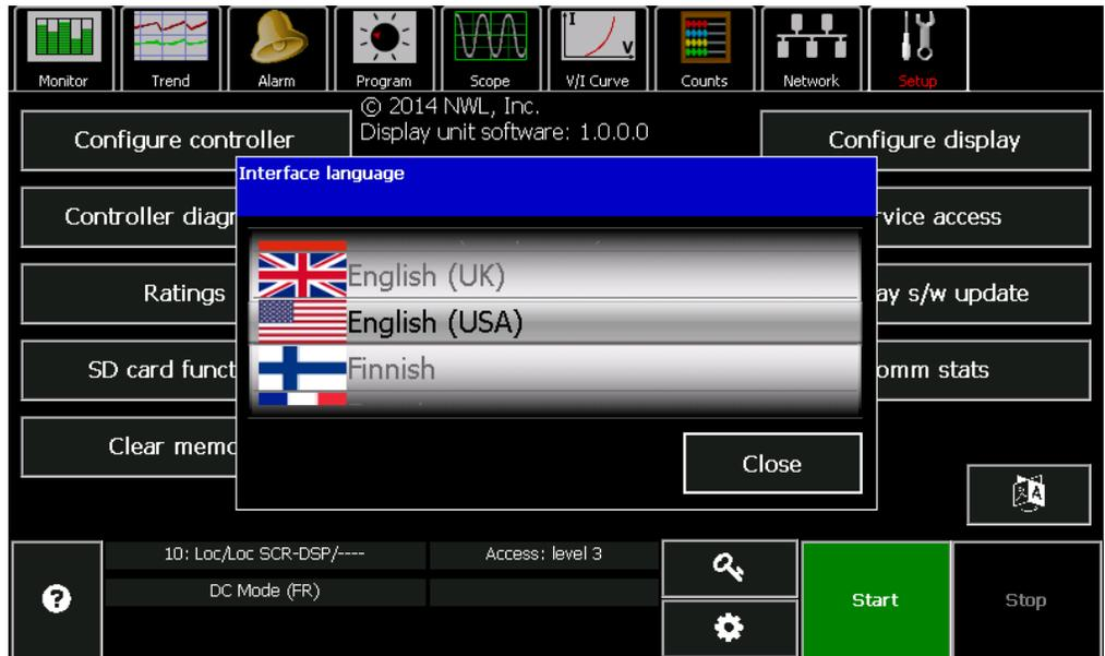
A roller display will appear. Pressing the country selection above or below the center highlighted area will cause the roller to go up or down one country at a time. Continue until the desired country is highlighted in the center of the roller. Press the **Close** button and the GDU will re-configure itself for that language. The re-configuration process involves a re-boot of the display will take a minute or so.
