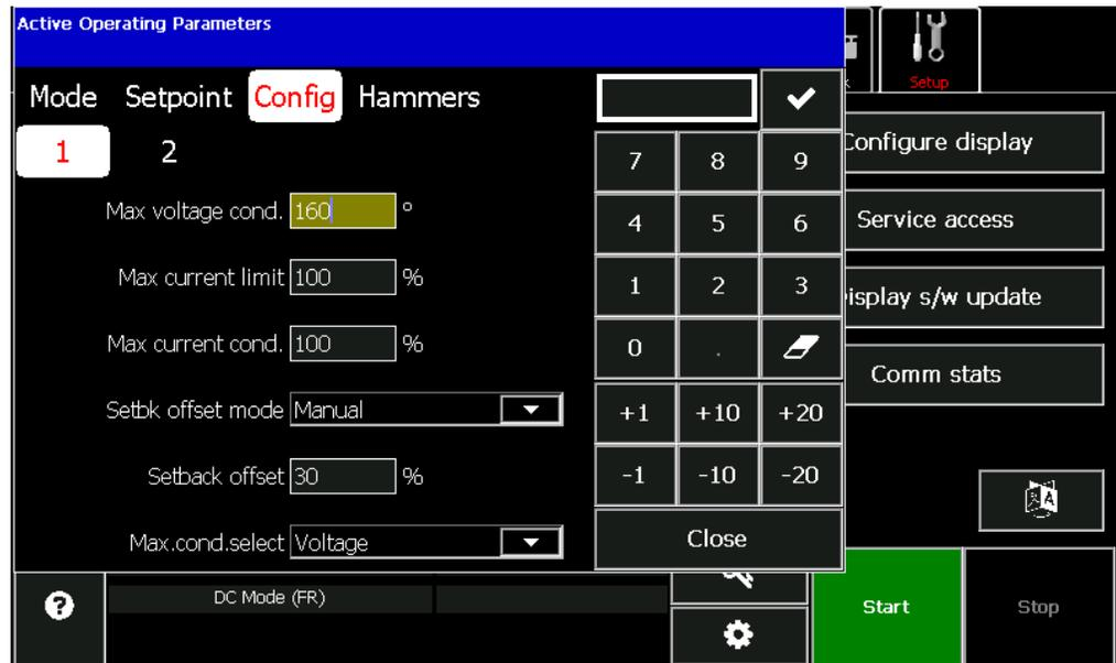
The ESP load will rarely let the T/R set's SCRs operate at their rated conduction angle of 160 degrees. Usually it will run at either a sparking level, a voltage limit, or a current limit.
