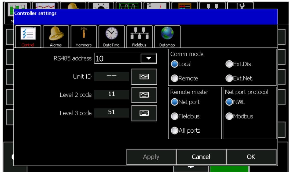
Use the *RS485 address* parameter to select a unique address from 10 through 99. Start with the *Comm mode* set to Local. Press OK.
