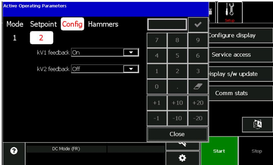
If the T/R does not have provisions for KV feedback, the GVC will calculate the secondary voltage based on the primary voltage reading.
