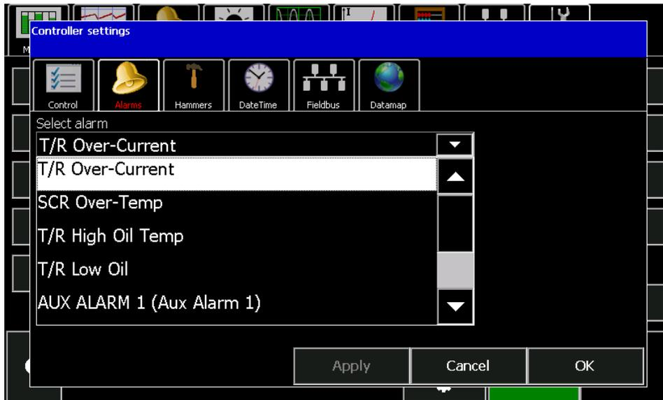
The alarms warn you of serious threats to precipitator operation, including potential damage to the T/R set. They are discrete alarms from external devices that are wired into the appropriate alarm input. The logic for each alarm must be configured.
