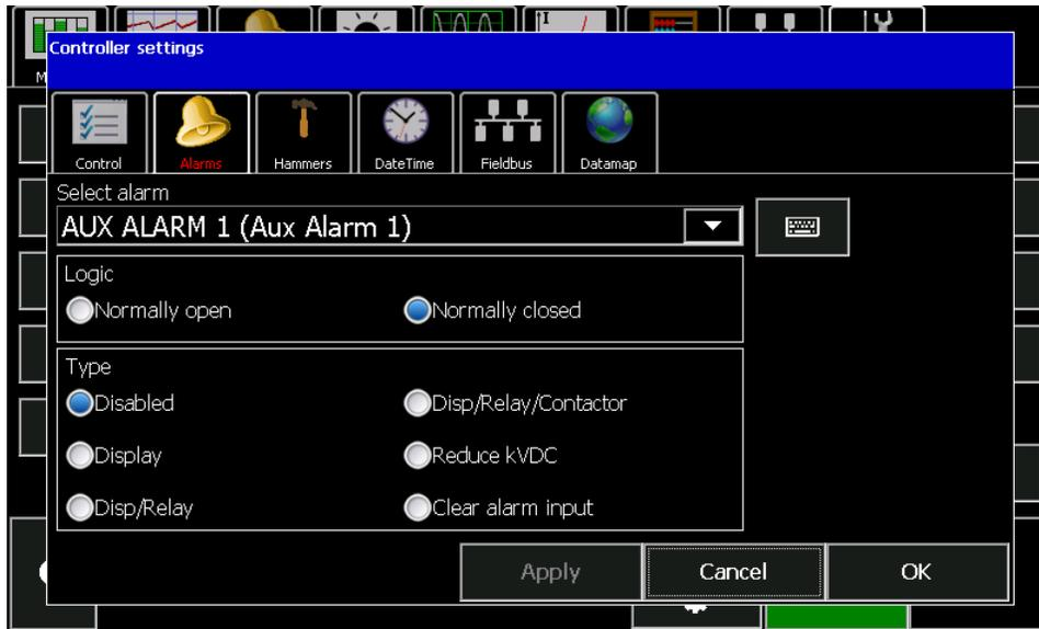
To advance through the auxiliary alarm configuration pages select the appropriate one from the pulldown list. By default, auxiliary alarms are displayed as numbers: *Aux Alarm 1*, *Aux Alarm 2*, etc. You can set them up to display as actual names.
