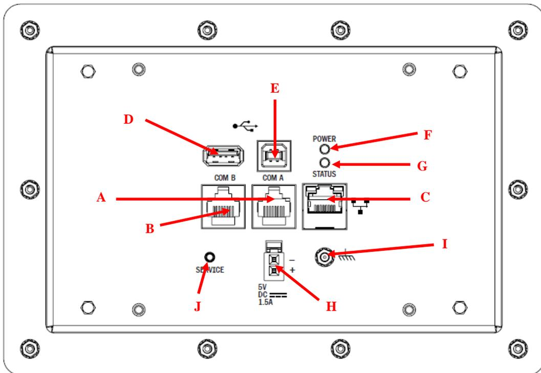
A - Com A: RS-485 port to be used for communicating with the GVC control. Display is powered by the 5 VDC within this cable.
