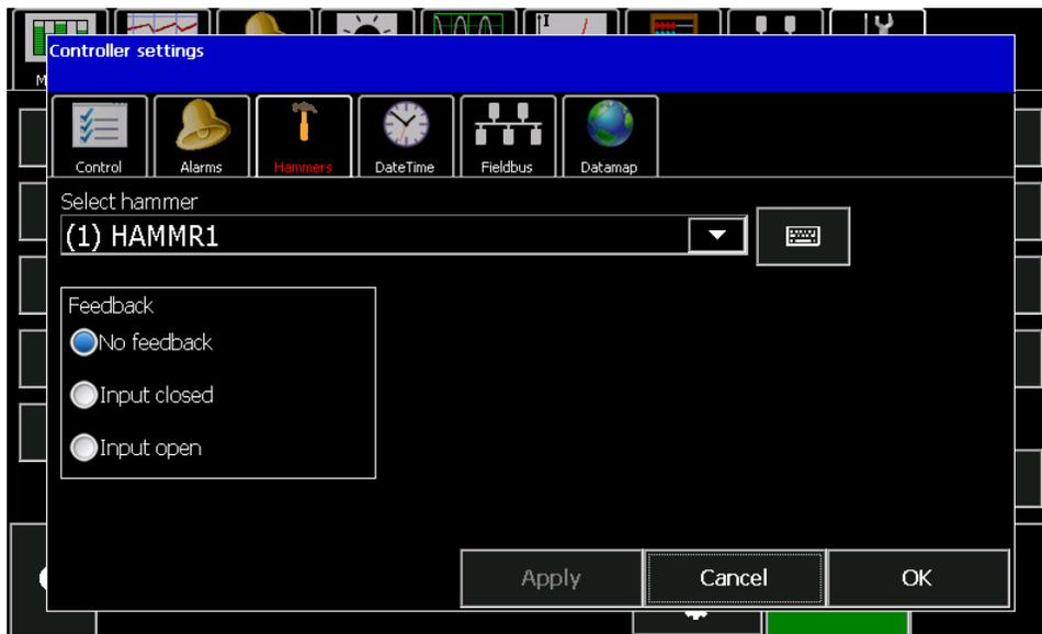
Start by selecting the appropriate hammer output from the **Select hammer** pulldown list. To give each hammer output a unique but specific ID, press the keyboard icon
