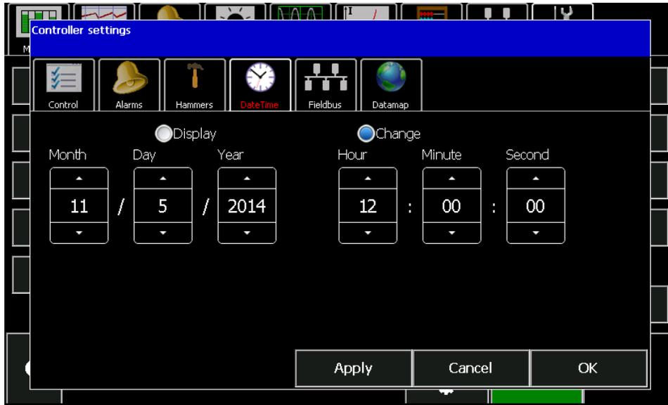
To edit the date or time, press the *Change* button then use the raise or lower arrows to enter the proper values. Press the *Apply* button when complete.
