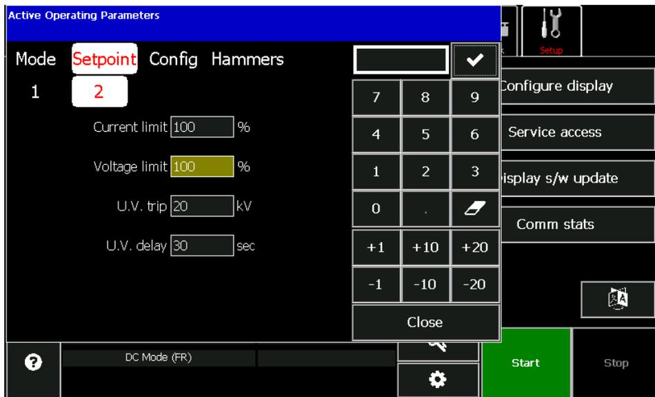
Highlight the U.V.Trip parameter value by touching it. Using the keypad on the right side of the screen press 0 and then press the
