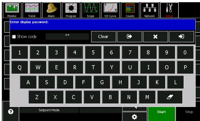
3. Type the password for the desired level of access. The default code for configuring the system is 51.
