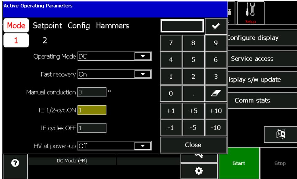
Using the pull down button next to the **Operating Mode** parameter, select *Manual* mode. Press the **Close** button.
