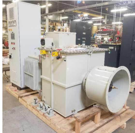
Figure 2: Contoller and HV tank for 3 phase SCR-CLR-TR system with approximatley 30% system reactance. Rated 70kVdc at 1000 mAdc.
