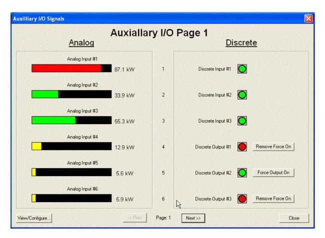
When viewing a particular Aux I/O page, clicking on the '<<Prev' or 'Next>>' buttons enables the user to navigate to alternate pages. If one of the Discrete signals is configured for a Discrete OUTPUT, a toggle button will be displayed allowing the user to force the respective output ON or remove the Force On condition if it already exists.
