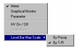
The next two items may be disabled, or grayed-out, if you do not have appropriate access to the functions to toggle the HV status of a Power Supply or to clear alarms.
