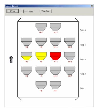
Hopper icons are divided into two sections. A Hi Hi Input is represented by the coloration of the top half of the hopper icon, while the Hi Input is represented by the bottom half.
