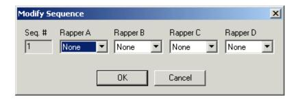
Select the rappers you wish to fire simultaneously, for this sequence. You may make up to four selections. Select *None* to indicate no rapper selection.
