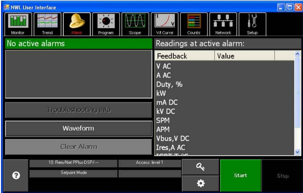
Pressing the “Waveform” button will upload and display the previous alarms waveform data.
