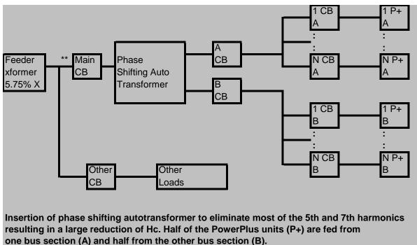
\*\* Point of Common Coupling at which Voltage Distortion is Measured. Max. kW load for THDv = 5% is 80% to 90% of feeder
