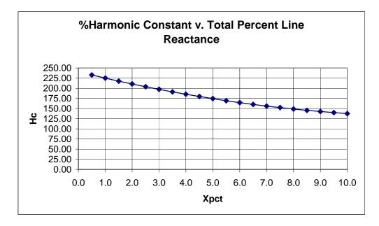
Please note that the horizontal scale in the above graph is for total percent reactance, which includes cable reactance and line reactors as well as the short circuit impedance of the 480 VAC feeder transformer. It is important to note that all of the preceding analysis is based on no power factor capacitors being on the feeder system. Once power factor capacitors are introduced, harmonic resonances can be setup and the analysis becomes more complex.
