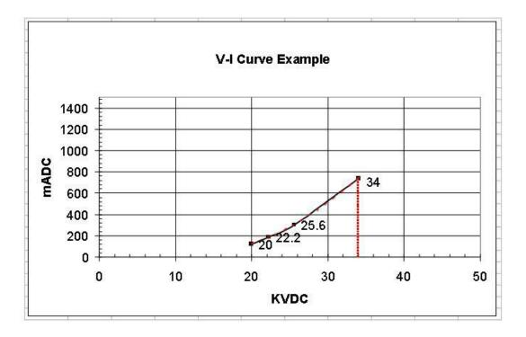
The slope of this curve will determine how much additional current will exist as the kVdc increases. If the V-I curve is very steep, large increases in mAdc will occur. If it is not steep, small increases in mAdc will occur. If the unit is sparking, it can be expected that that kVdc will approach the value of the kVpeak that was measured in
