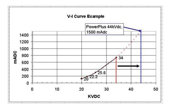
The original T/R was operating at 34 kVdc and 750 mAdc. The replacement PowerPlus will be expected to operate at about 44 kVdc and 1500 mAdc. In this example the 70 kVdc, 1500 mAdc, 105 kW PowerPlus size should be selected.
