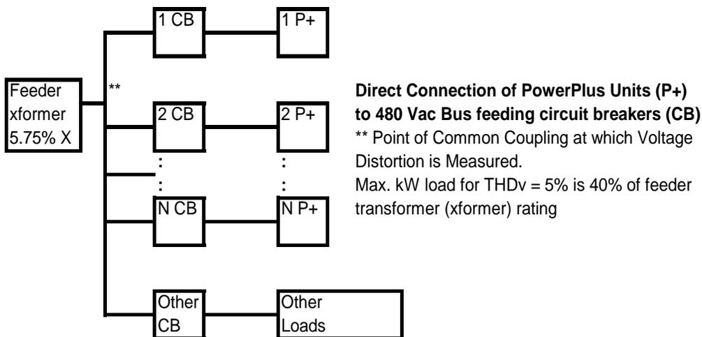
Inserting 3% line reactance (a three phase line reactor) between the feeder transformer and the 480 VAC bus feeding the PowerPlus units allows the kW load to be increased to 50% of the transformer rating while still maintaining the 5% THD<sub>v</sub> level.
