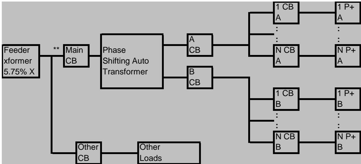
**Insertion of phase shifting autotransformer to eliminate most of the 5th and 7th harmonics resulting in a large reduction of Hc. Half of the PowerPlus units (P+) are fed from one bus section (A) and half from the other bus section (B).**
